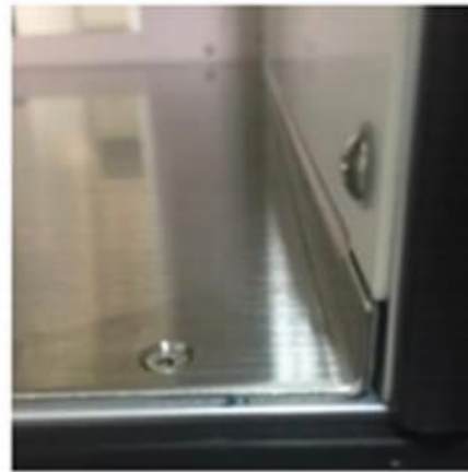
SUS interior floor with R for easy cleaning
